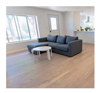
Wood is a natural substance and has pores that will allow it to expand and contract with humidity and temperature changes. In solid wood, it is difficult to install wood planks that are over 4" wide because the expansion and contraction will cause gapping and "cupping" when the seasons change. The wider the wood, the more expansion and contraction you can expect. That's where engineered wood is beneficial.
